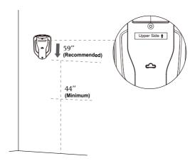
4. To store, hang the hand vacuum on the wall mount. Align the slot on the bottom of the hand vacuum with the protrusion on the wall mount as shown in the picture below.
