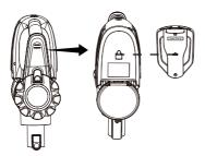
5. Insert the 2-in-1 combination tool into the right slot on top of the wall mounting bracket for convenient storage. Insert the crevice tool into the left slot.
