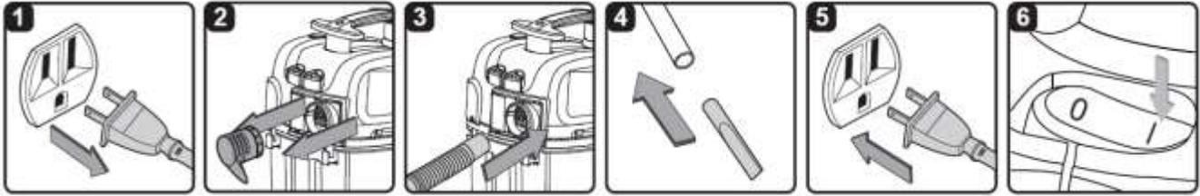
This Wet/Dry Vac has blowing capabilities only when the hose is inserted into the blowing port. To use the blower feature follow the instructions listed.
